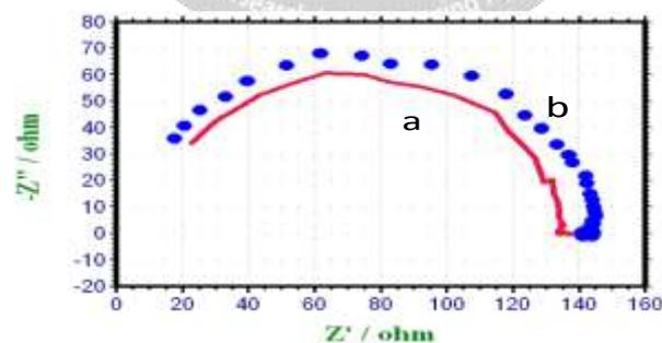
Fig 2 AC impedance spectra of carbon steel immersed in various test solutions (Nyquist plots)
