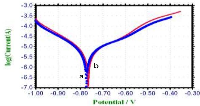
Fig 1. Polarization curves of carbon steel immersed in various test solutions
