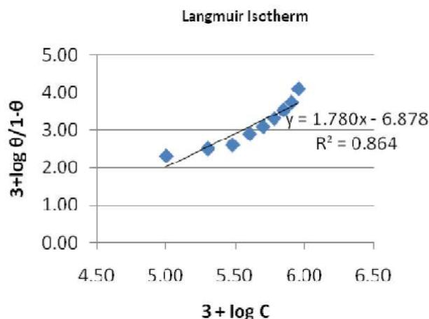
**Figure 2.** Langmuir adsorption isotherm for mild steel corrosion inhibition in 1 N HCl, using *Commelina benghalensis* leaves extract.
