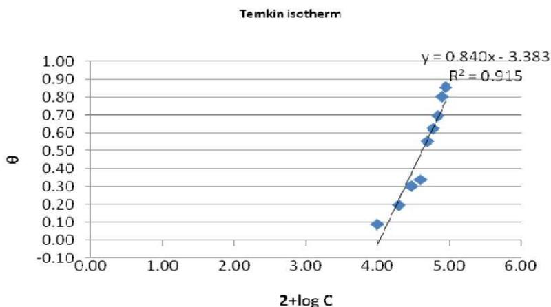
**Figure 5.** Temkin adsorption isotherm for mild steel corrosion inhibition in 0.5 M H<sub>2</sub>SO<sub>4</sub>, using *Commelina benghalensis* leaves extract.
