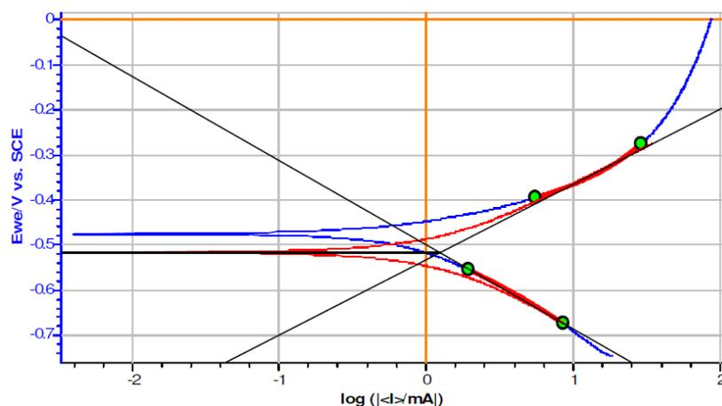
**Figure 14.** Potentiometric polarization curve for 0.5 M H<sub>2</sub>SO<sub>4</sub> medium, in the presence of 100 ppm concentration of *Commelina benghalensis* leaves extract.
