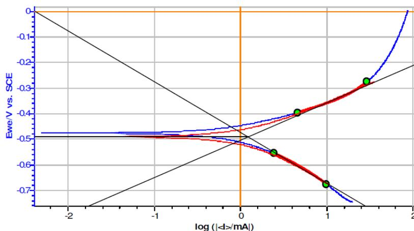
**Figure 13.** Potentiometric polarization curve for mild steel in 0.5 M H<sub>2</sub>SO<sub>4</sub>.
