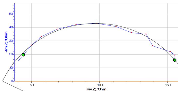
**Figure 21.** Impedance diagram for mild steel in 0.5 M H<sub>2</sub>SO<sub>4</sub> medium, in the presence of 900 ppm concentration of *Commelina benghalensis* leaves extract.
