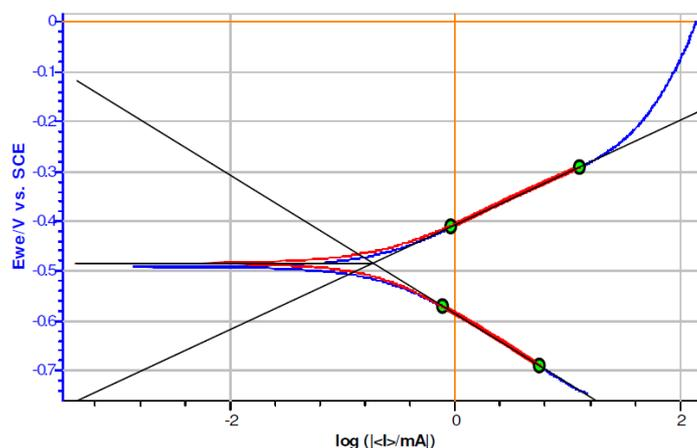
**Figure 10.** Potentiometric polarization curve for 1 N HCl medium.
