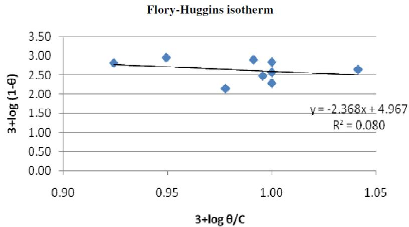
**Figure 7.** Flory-Huggins adsorption isotherm for mild steel corrosion inhibition in 0.5 M H<sub>2</sub>SO<sub>4</sub>, using *Commelina benghalensis* leaves extract.
