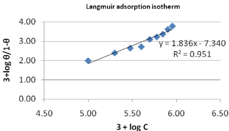
**Figure 3.** Langmuir adsorption isotherm for mild steel corrosion inhibition in 0.5 M H<sub>2</sub>SO<sub>4</sub>, using *Commelina benghalensis* leaves extract.
