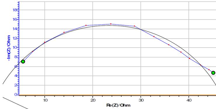
**Figure 18.** Impedance diagram for mild steel in 1 N HCl medium, in the presence of 900 ppm concentration of *Commelina benghalensis* leaves extract.
