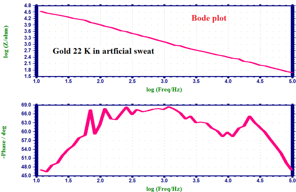
Figure 10. Bode plot of Gold 22 K alloy immersed in artificial sweat
