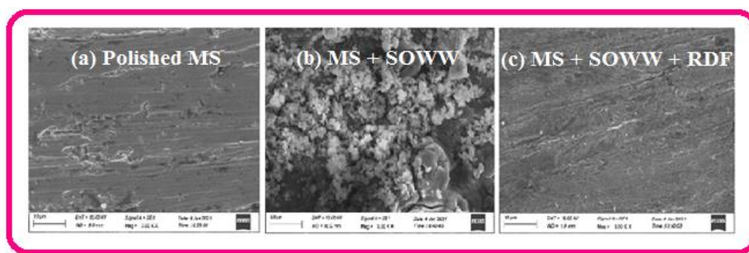
Figure 3. SEM image of (a) polished mild steel; (b) mild steel immersed in SOWW (blank); (c) mild steel immersed in SOWW containing inhibitor (RDF).
