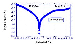
**Figure 2:** Polarization curve of 18 K Goldimmersedin artificial saliva in the presence of Gelusil
