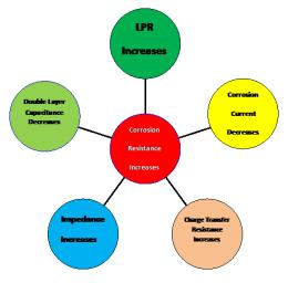
Scheme B. Correlation among corrosion resistance and corrosion parameters
