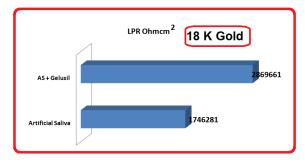
**Figure 3:** Comparison of linear polarization resistance values of 18 K Gold in artificial salivain the absence and presence of Gelusil
