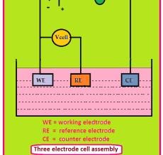
Scheme A. Three electrode cell assembly
