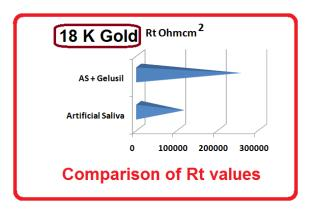
**Figure 8:** Column chart of charge transfer values of 18 K Gold in the absence and presence of Gelusil
