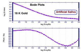
**Figure 4:** AC impedance spectrum of 18 K Goldimmersed in Artificial Saliva
