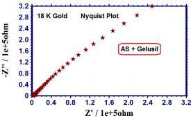
**Figure 6:** AC impedance spectrum of 18 K Gold immersed in Artificial Saliva (Nyquist Plot)
