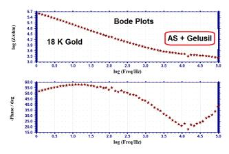
**Figure 7:** AC impedance spectra of 18 K Gold immersed in Artificial Saliva in the presence of Gelusil (Bode Plots)
