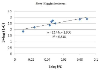
**Figure 6.** Flory-Huggins adsorption isotherm for mild steel corrosion inhibition in 1 N HCl, using *Commelina benghalensis* leaves extract.
