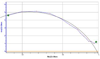
**Figure 20**. Impedance diagram for mild steel in 0.5 M H<sub>2</sub>SO<sub>4</sub> medium, in the presence of 100 ppm concentration of *Commelina benghalensis* leaves extract.
