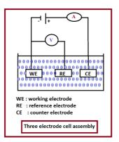
Scheme 1. Three electrodes cell.
