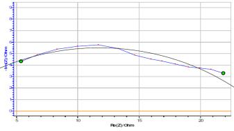
**Figure 17.** Impedance diagram for mild steel in 1 N HCl medium, in the presence of 100 ppm concentration of *Commelina benghalensis* leaves extract.
