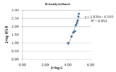
**Figure 9.** El-Awady adsorption isotherm for mild steel corrosion inhibition in 0.5 M H<sub>2</sub>SO<sub>4</sub>, using *Commelina benghalensis* leaves extract.
