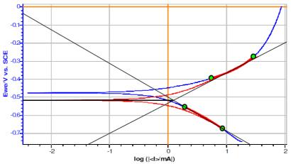
**Figure 14.** Potentiometric polarization curve for 0.5 M H<sub>2</sub>SO<sub>4</sub> medium, in the presence of 100 ppm concentration of *Commelina benghalensis* leaves extract.
