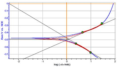
Figure 13. Potentiometric polarization curve for mild steel in 0.5 M H<sub>2</sub>SO<sub>4</sub>.
