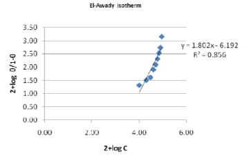
**Figure 8.** El-Awady adsorption isotherm for mild steel corrosion inhibition in 1 N HCl, using *Commelina benghalensis* leaves extract.
