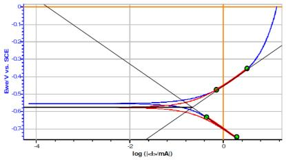
**Figure 15.** Potentiometric polarization curve for 0.5 M H<sub>2</sub>SO<sub>4</sub> medium, in the presence of 900 ppm concentration of *Commelina benghalensis* leaves extract.
