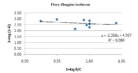
**Figure 7.** Flory-Huggins adsorption isotherm for mild steel corrosion inhibition in 0.5 M H<sub>2</sub>SO<sub>4</sub>, using *Commelina benghalensis* leaves extract.
